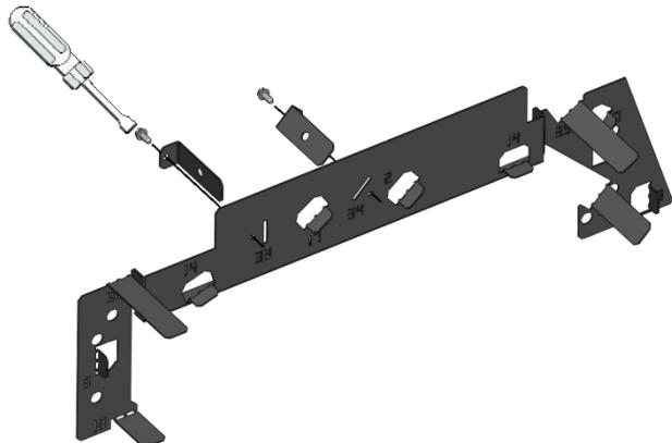
9. Install the rear stone grid assembly by sliding it under the rear light deflector. The grid assembly should rest over the two burner tabs as shown below.
