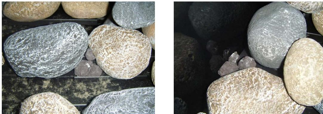
3. Re-apply the rock wool over the ember chunks along the front burner and between the two front stones for a natural look.
