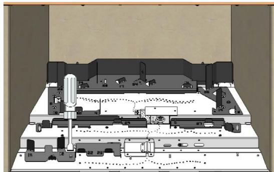
13. Install the front right stone grid plate using a 10-24 nut. Keep the grid plate tight against the front burner's front edge.
