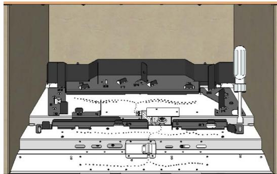
12. Install the front left stone grid plate using a 10-24 nut. Keep the grid plate tight against the front burner's front edge.
