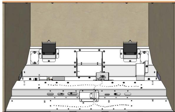
3. Install the rear light deflector using the screws removed in the previous step.
