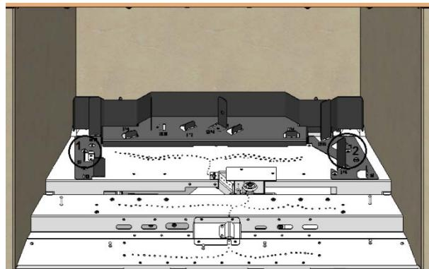
10. Install the center left stone grid plate using a 10-24 nut. Keep the grid plate tight against the rear burner's front edge.
