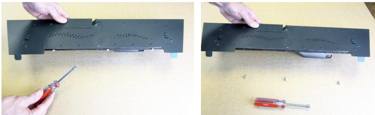
5. Attach the rear air deflector to the rear burner with the screws removed in the previous step.
